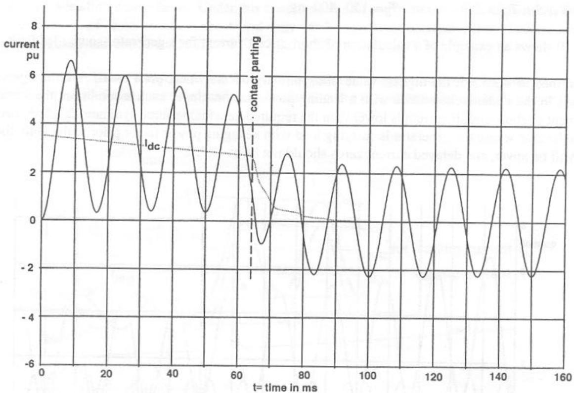
FIGURE 2. Short-circuit Current with Delayed Current Zeroes [1]
