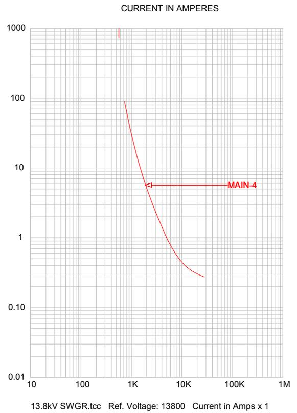
Fig. 4 Time Current Characteristics of the main protective devices in sample systems 1 through 4
