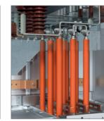
Ample cable termination provision is provided up to 6 single core cables per phase to enter the bottom of the switchgear and are terminated with compression lugs onto copper tails provided in the bottom of each panel.
