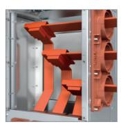
Busbars are totally enclosed in their own earthed metal compartment which vents into the arc chamber. Fully insulated along their entire length, the bushars are type tested for ratings up to 3150A, 31.5kA for 3 seconds. Epoxy mouldings segregate switchgear sections.
