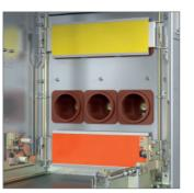
Individually operated automatic earthed metal shutters for both the Line (busbar) and Load (cable) connections can be padlocked in the closed position. When the breaker is in Test or Disconnect positions the shutters automatically close to prevent accidental contact
