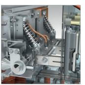
The earth switch is operated from the front of the switchgear, with mechanical indicators to show the switch position. A window allows direct viewing of the earth switch position. The earth switch is mechanically interlocked with the circuit breaker or contactor truck such that it can only be closed when truck is in the Test/Disconnect position. The circuit earth switch can be mechanically interlocked
